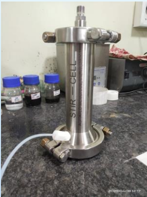
High pressure filtration unit
