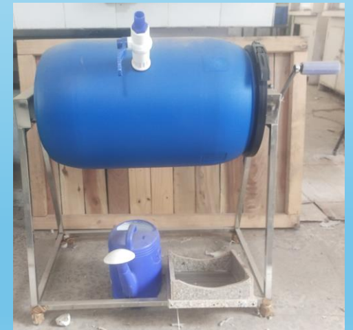
Rotatory anerobic digester
