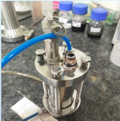
Low pressure filtration unit
